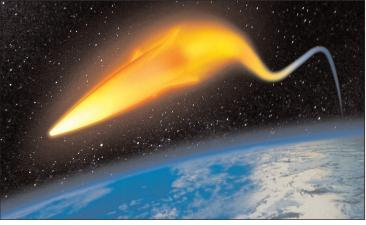
The highly predictable flight paths and high altitudes of non-manoeuvring ballistic missiles make them much easier to detect and track. In contrast, hypersonic missiles can fly as little as 30 to 50 km above the Earth's surface or even lower, which means that, because of the curvature of the earth, they may be below areas that are effectively covered by today's radar warning architecture.
